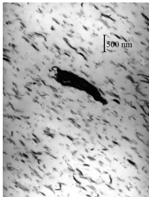
Figure 6. Transmission electron microscopy (TEM) image of PLA nanocomposite containing 3 wt % clay.
